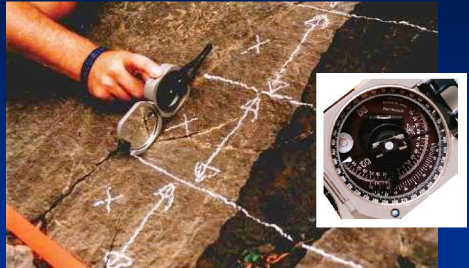
Measuring Dip Angle
