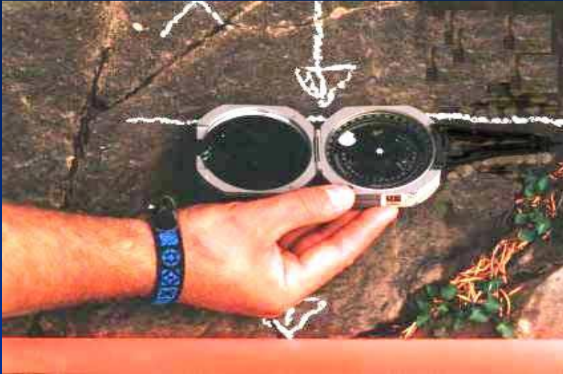
Measuring Strike Azimuth
