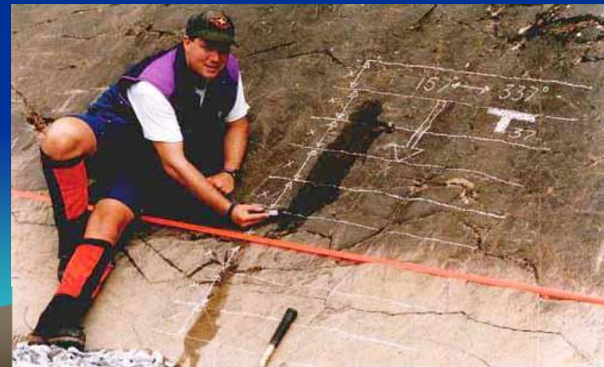
Completed Strike and Dip Measurement
