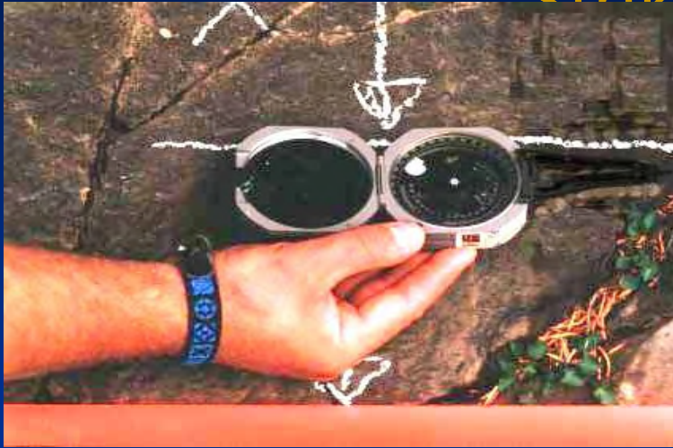
Measuring Strike Azimuth
