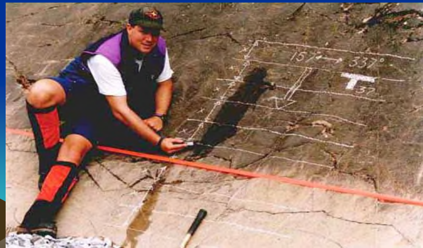
Completed Strike and Dip Measurement
