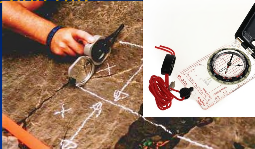
Measuring Dip Angle
