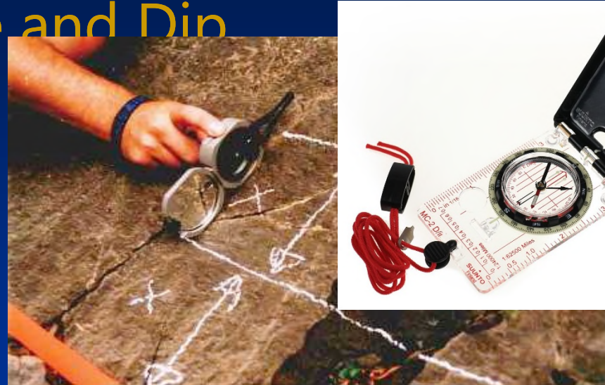
Measuring Dip Angle
